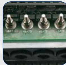
The DC connection on threaded rods is particularly robust and practical due to the available space.
